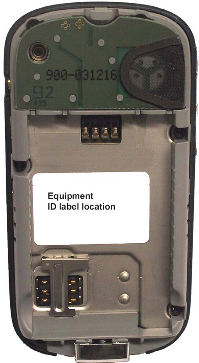
Rear view with battery removed to show equipment ID label
