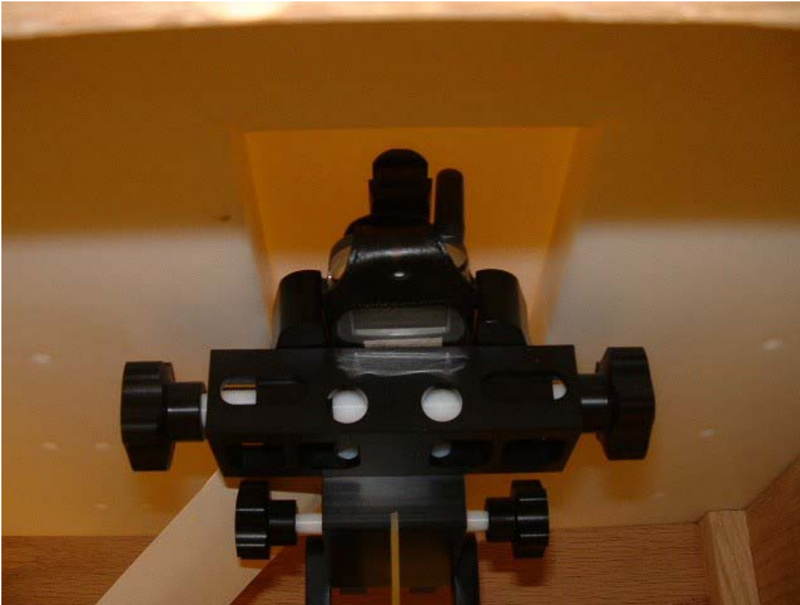
Figure 8. Phone against the flat phantom with leather pouch (Body worn position)
