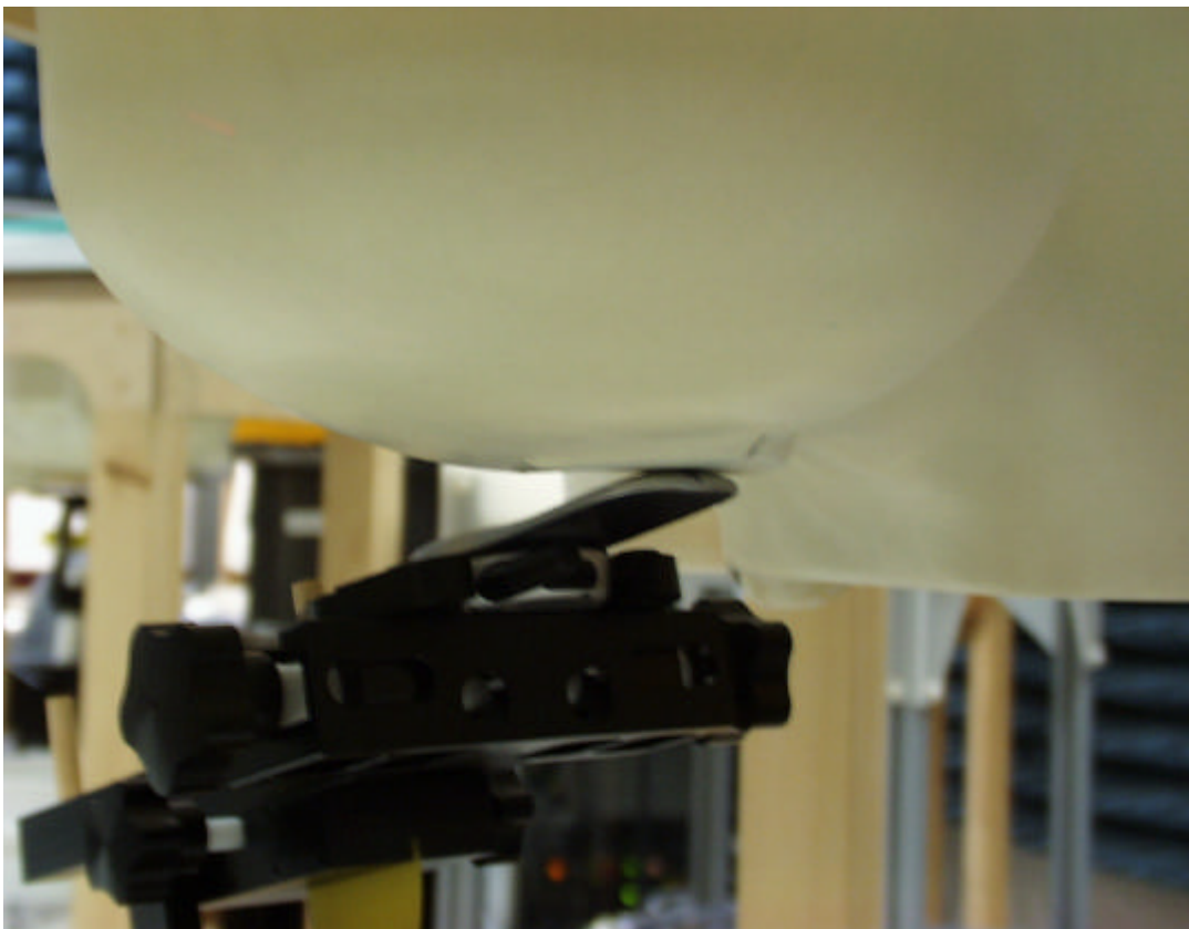
Figure 15. Phone Against the SAM Head Phantom 15° Tilt Position (Back View)
