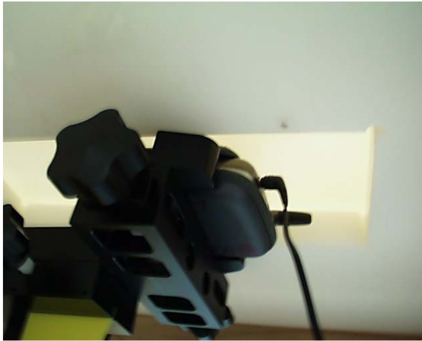
Figure 10. Phone in pouch under flat phantom (Body Worn)
