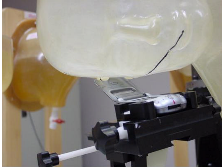
Figure1. Phone Against the Head in a 15° Tilt Position
