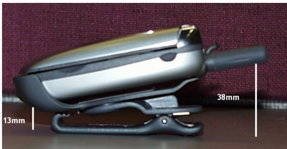
Figure 6. Separation Distance Provided by Phone in Belt Clip
