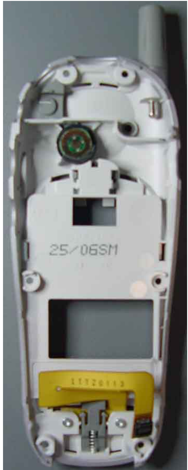
Rear Housing Internal View
