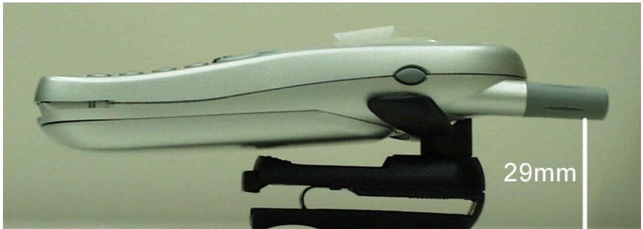
Figure 7. Proximity provided by Belt-clip
