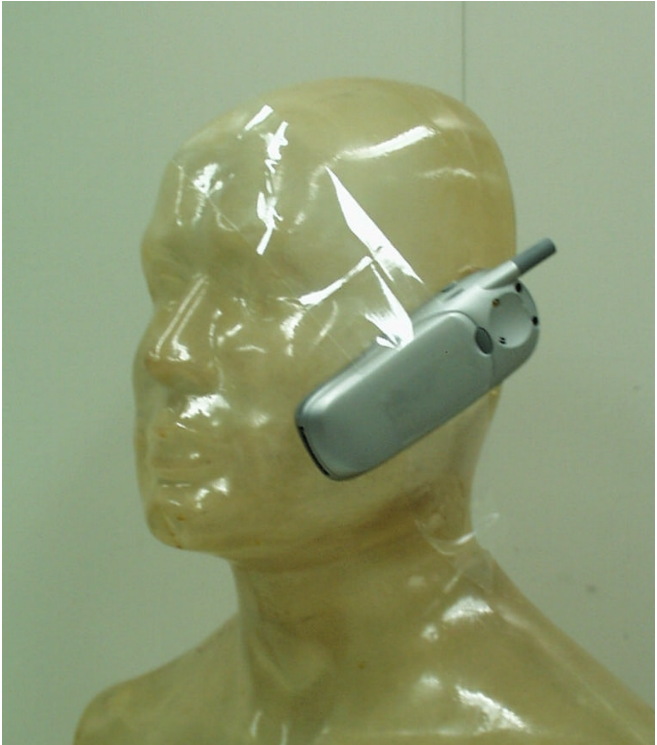
Figure 5. Phone against Phantom Head
