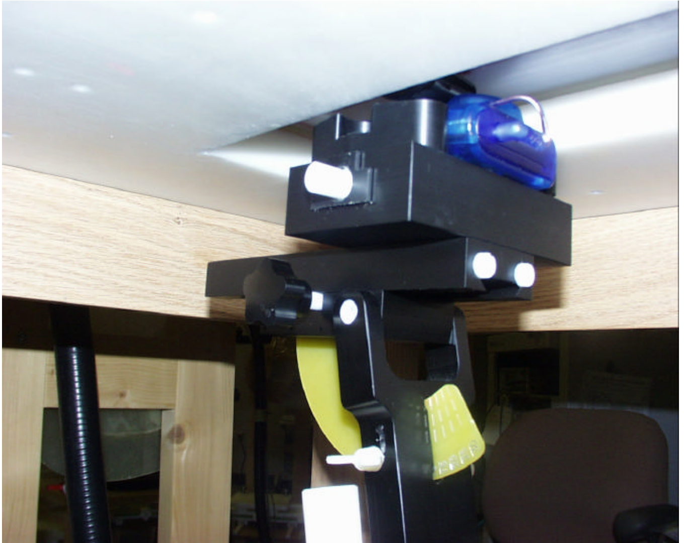
Figure 7. Body Worn Position of the Phone with the Phone clip Placed Under a Flat Phantom
