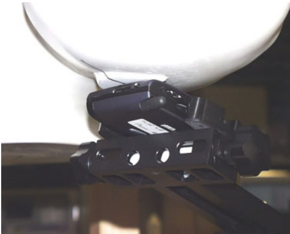
Figure 10. Phone in Cheek Touch Position with Speaker and Microphone Placed Against Phantom Head.
