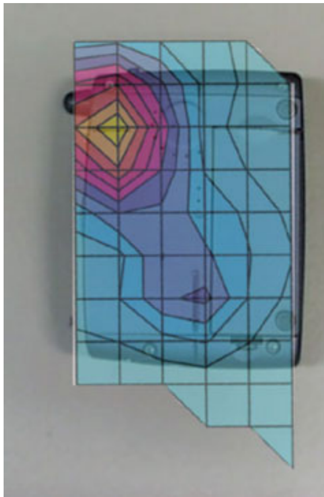
Figure 1. Typical Head Adjacent Contour Plot Overlaid on Bottom of Phone
