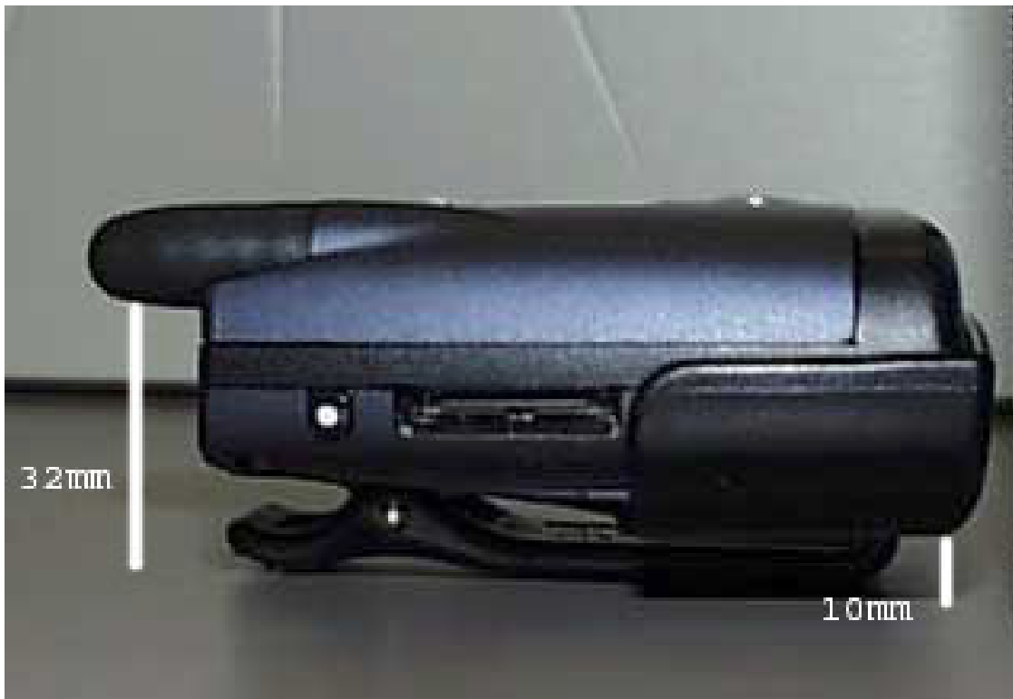
Figure 6. Separation Distances Provided from Body Worn Accessory
