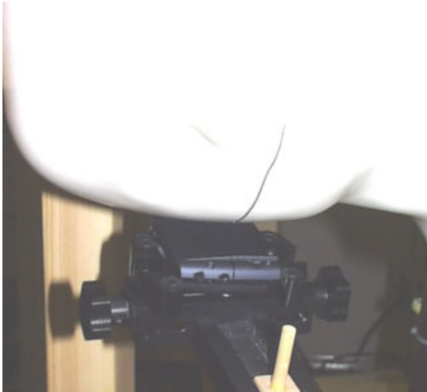
Figure 7. Phone in Cheek Touch Position with Speaker and Microphone Placed Against Phantom Head.
