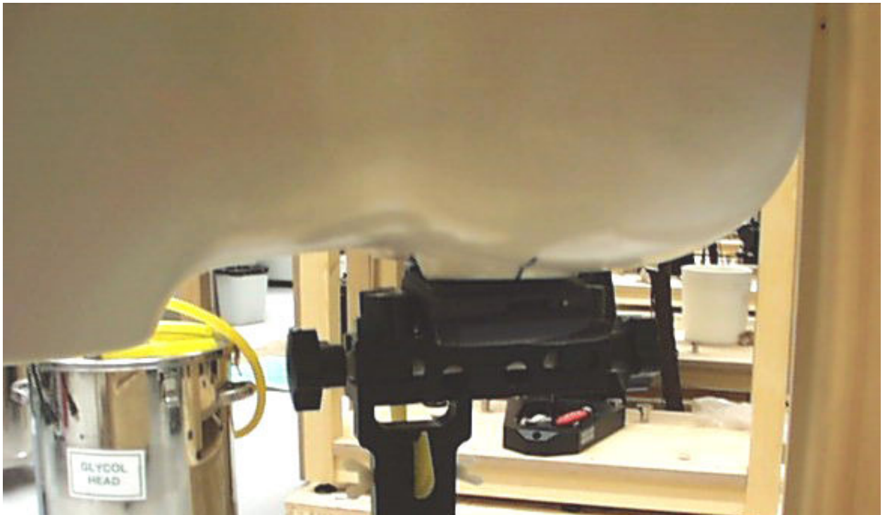
Figure 9. Phone in Cheek Touch Position with Speaker and Microphone Placed Against Phantom Head.
