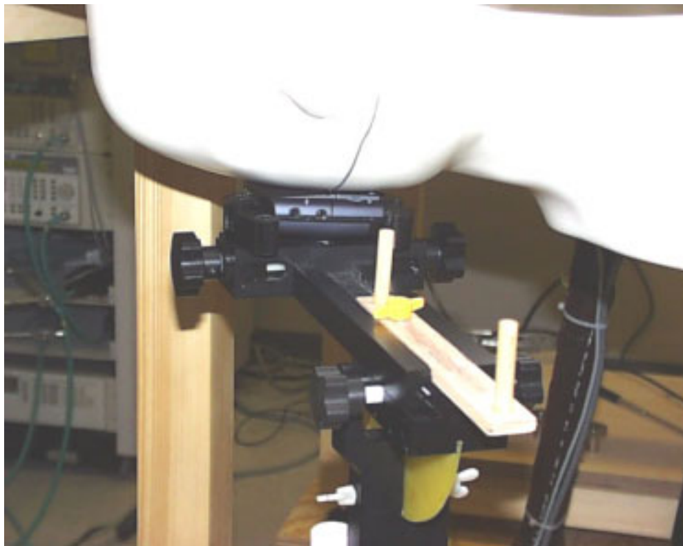
Figure 8. Phone in Cheek Touch Position with Speaker and Microphone Placed Against Phantom Head.
