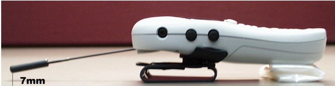
Figure 3. Separation Distances Provided by Belt-Clip with Antenna Extended
