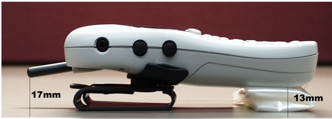
Figure 4. Separation Distances Provided by Belt-Clip with Antenna Retracted
