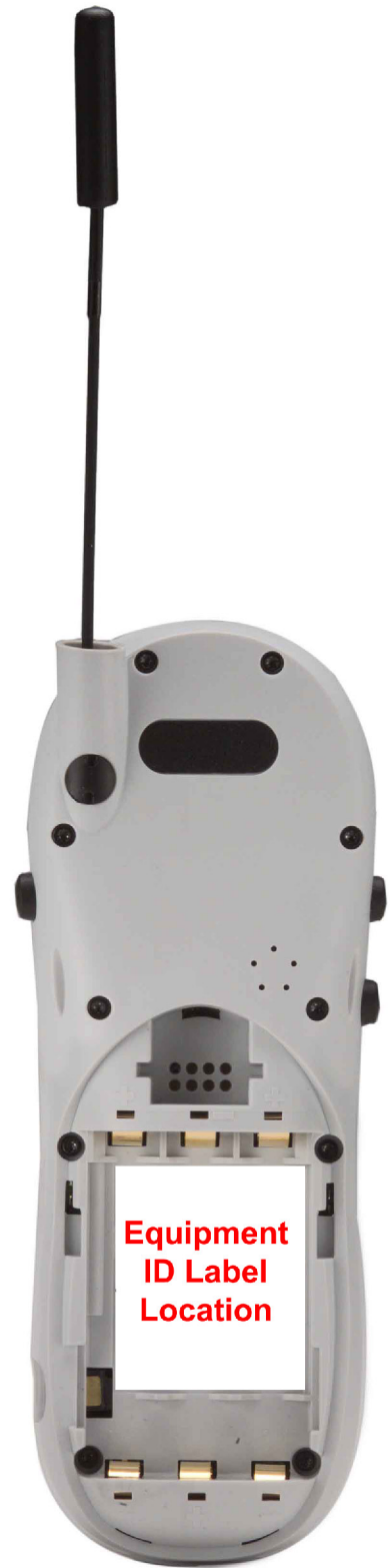
Back View Antenna Extended (Battery Removed to Show Equipment ID)
