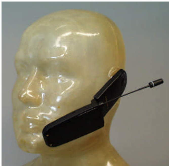
Figure 4. Phone against Phantom Head with Antenna Extended
