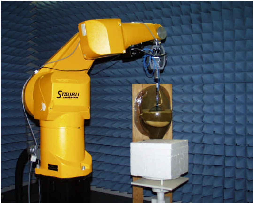
Figure 5. Dasy™ system with the Motorola Phantom.
