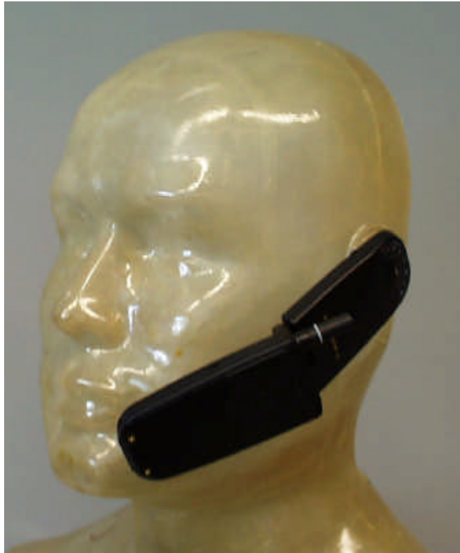
Figure 3. Phone against Phantom Head with Antenna Retracted
