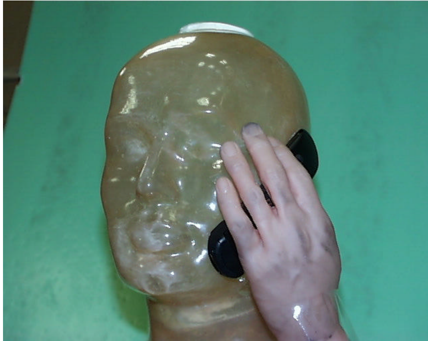
Figure 7. Simulated Hand Against Phantom Head.
