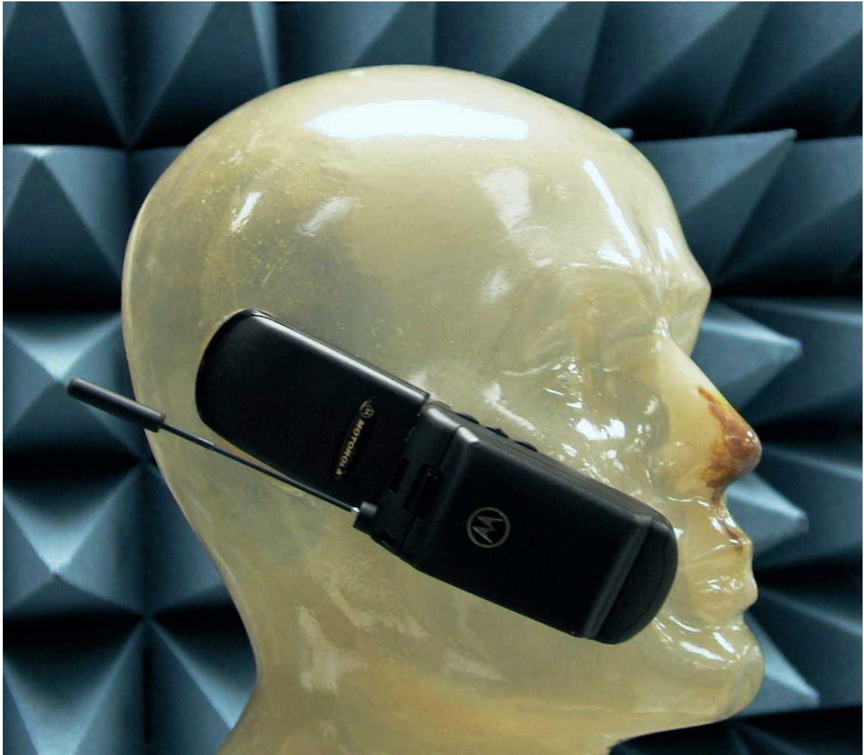
Figure 3. Phone against side of Phantom Head.
