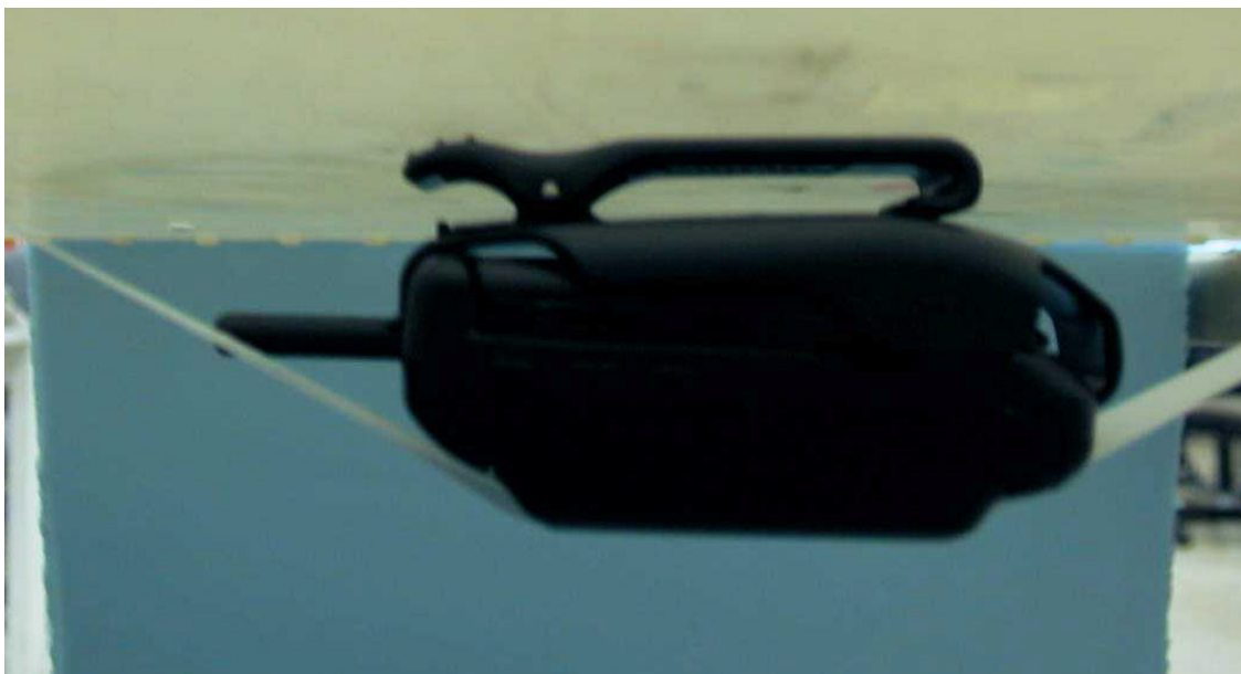
Figure 9. Phone In Supplied Belt Clip Against Phantom
