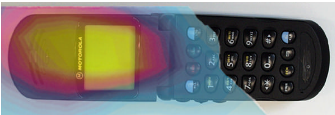
Figure 6. Digital Mode Contour Plot with Antenna Extended Overlaid on Face of Phone.
