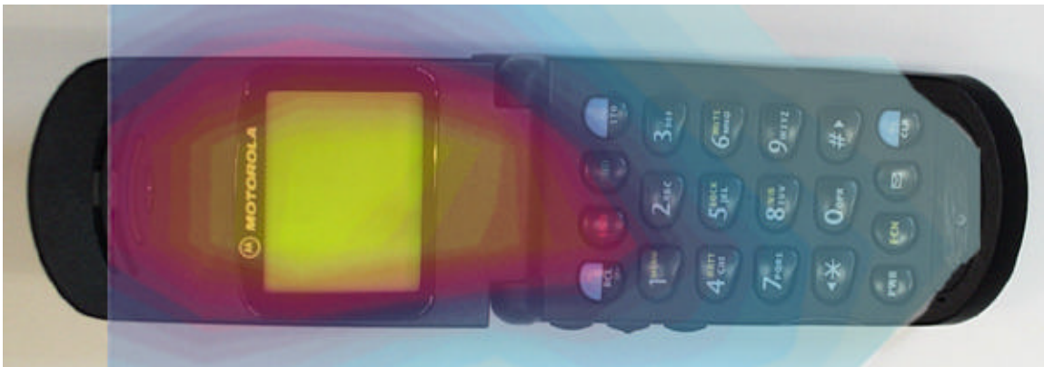
Figure 5. Analog Mode Contour Plot with Antenna Extended Overlaid on Face of Phone.
