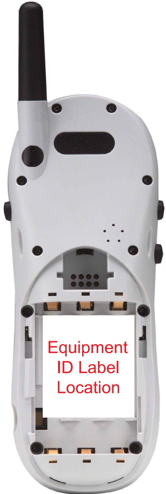
Back View (Battery Removed to Show Equipment ID)
