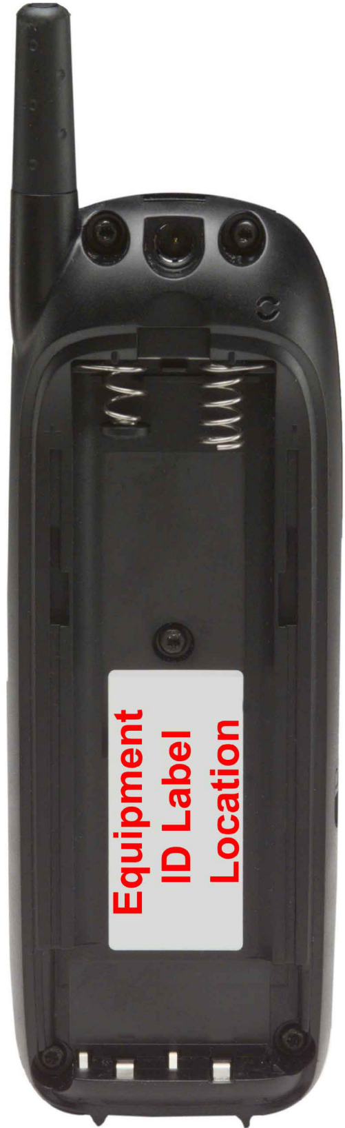
Back View (Battery Removed to Show Equipment ID)
