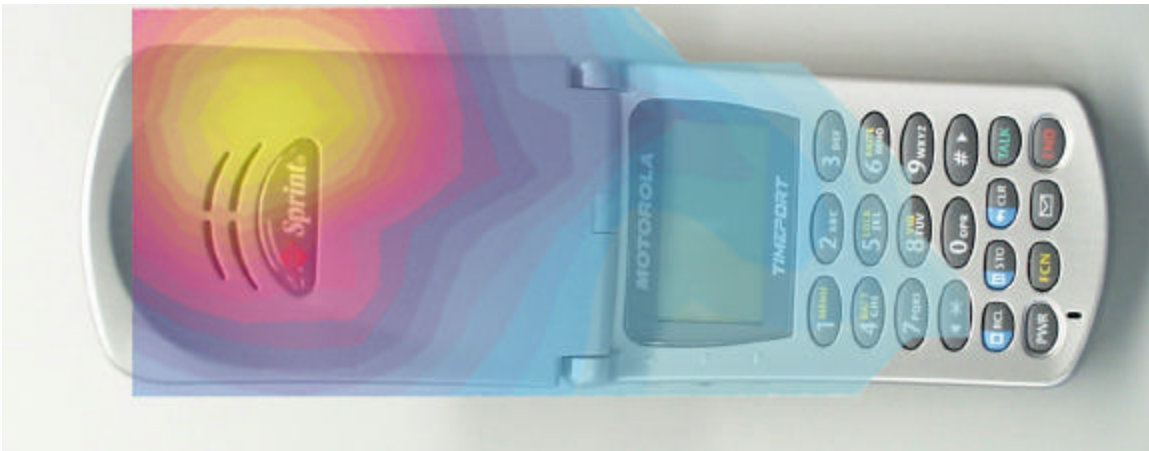
Figure 1. Contour Plot Overlaid on Face of Phone with Antenna Extended.
