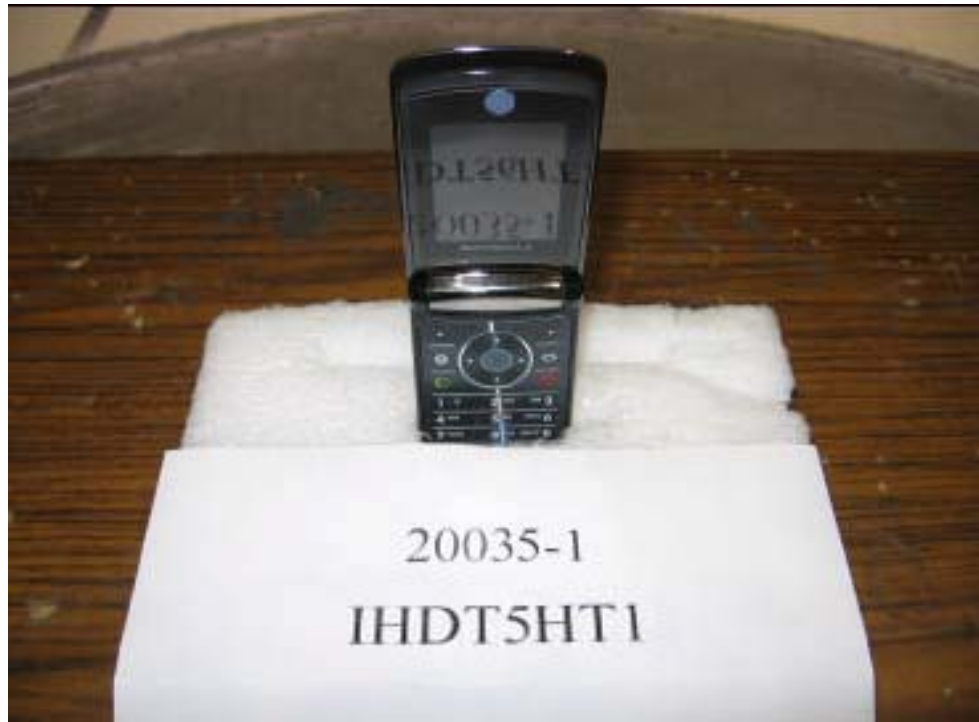
RADIATED EMISSIONS (X-AXIS)
