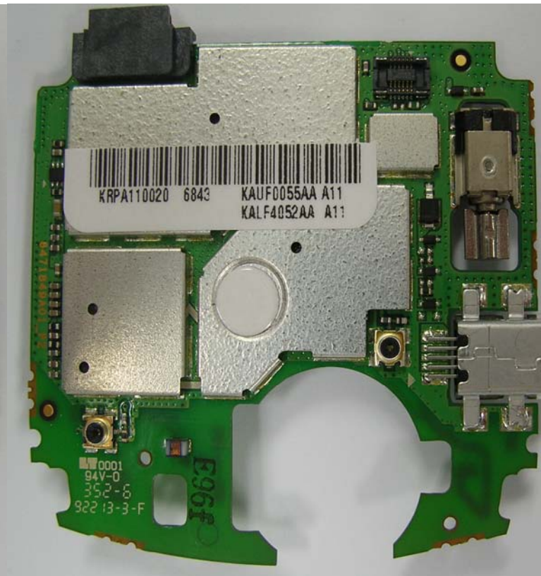
Main Board(Shield on)
