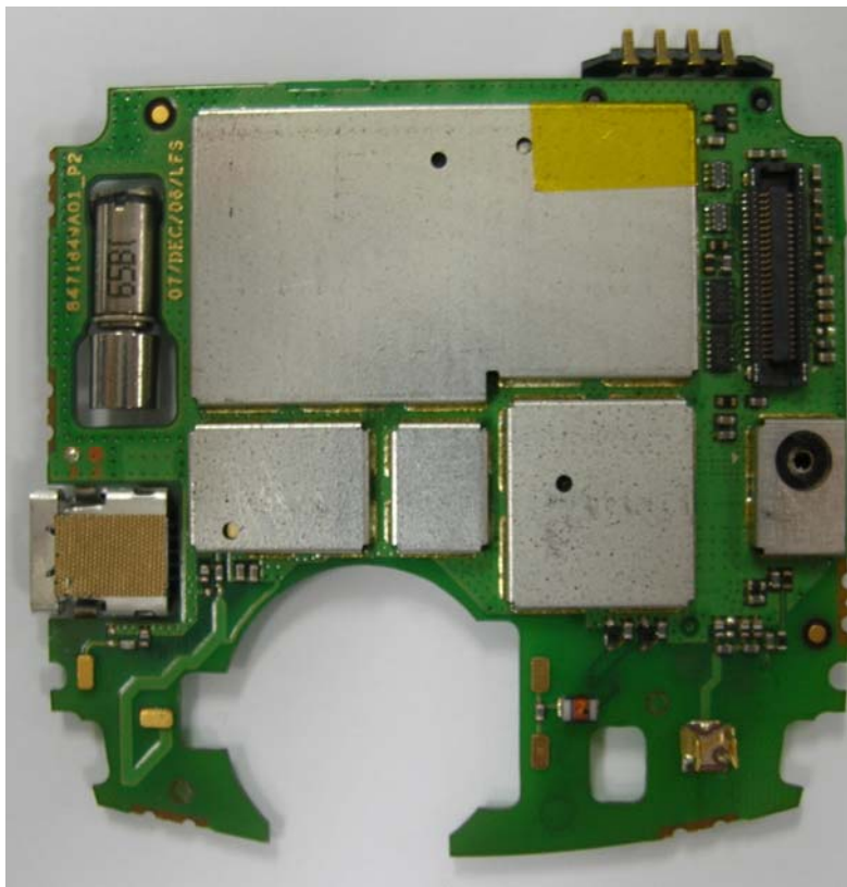
Main Board(shield on)
