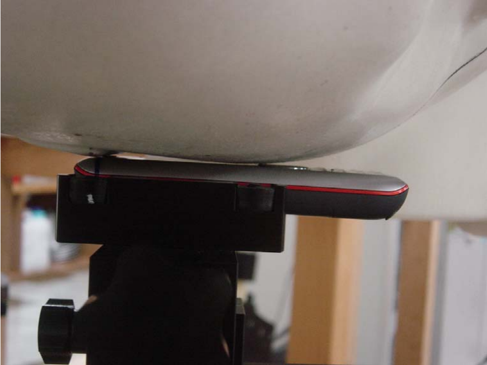
Figure 3. Phone against the Head Phantom (Cheek Touch)
