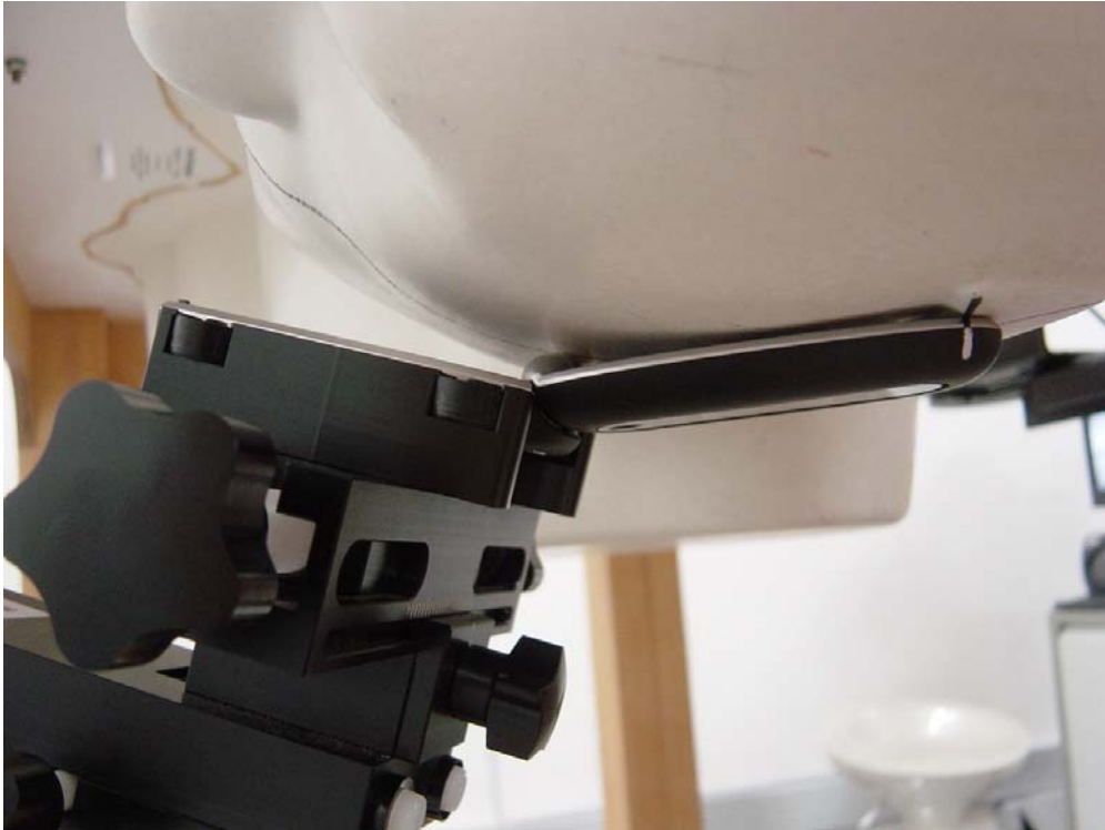
Figure 5. Phone Against the Head Phantom (Cheek Touch)
