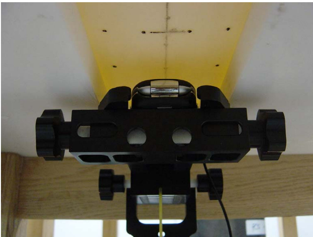
Figure 4. Phone Against the Flat Phantom
