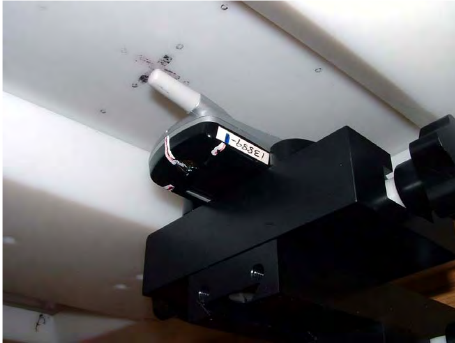
Figure 12. Phone in Against the Flat Phantom
