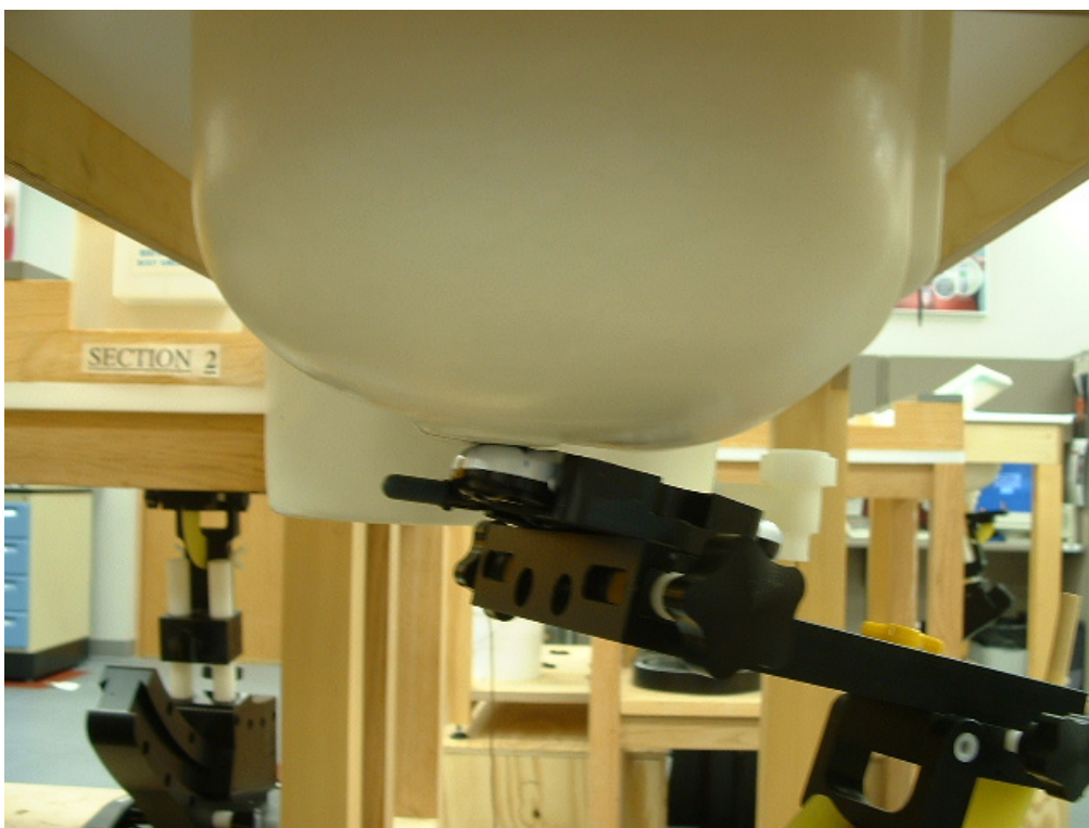
Figure 9. Phone against the Head 15° Tilt (Back View)
