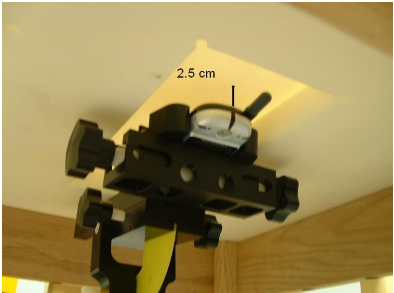
Figure10. Phone against the flat phantom 2.5 cm separation distance (Body worn position)
