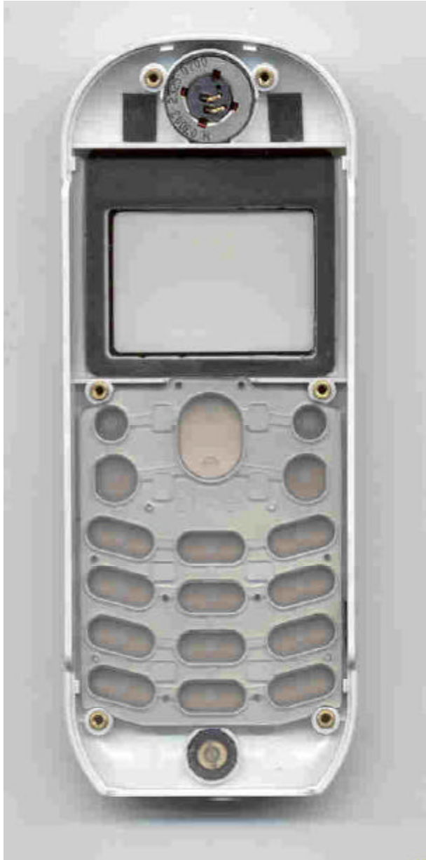
Inside the Front Housing
