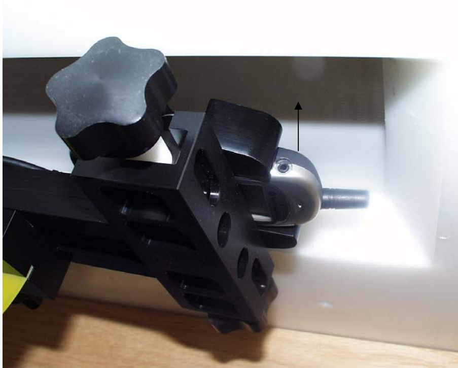
Figure 11. Back of Phone 1 inch away from Flat Phantom
