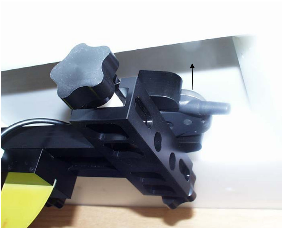
Figure 10. Front of Phone 1 inch away from Flat Phantom
