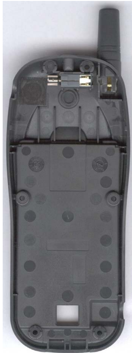
Rear Housing (Internal View)
