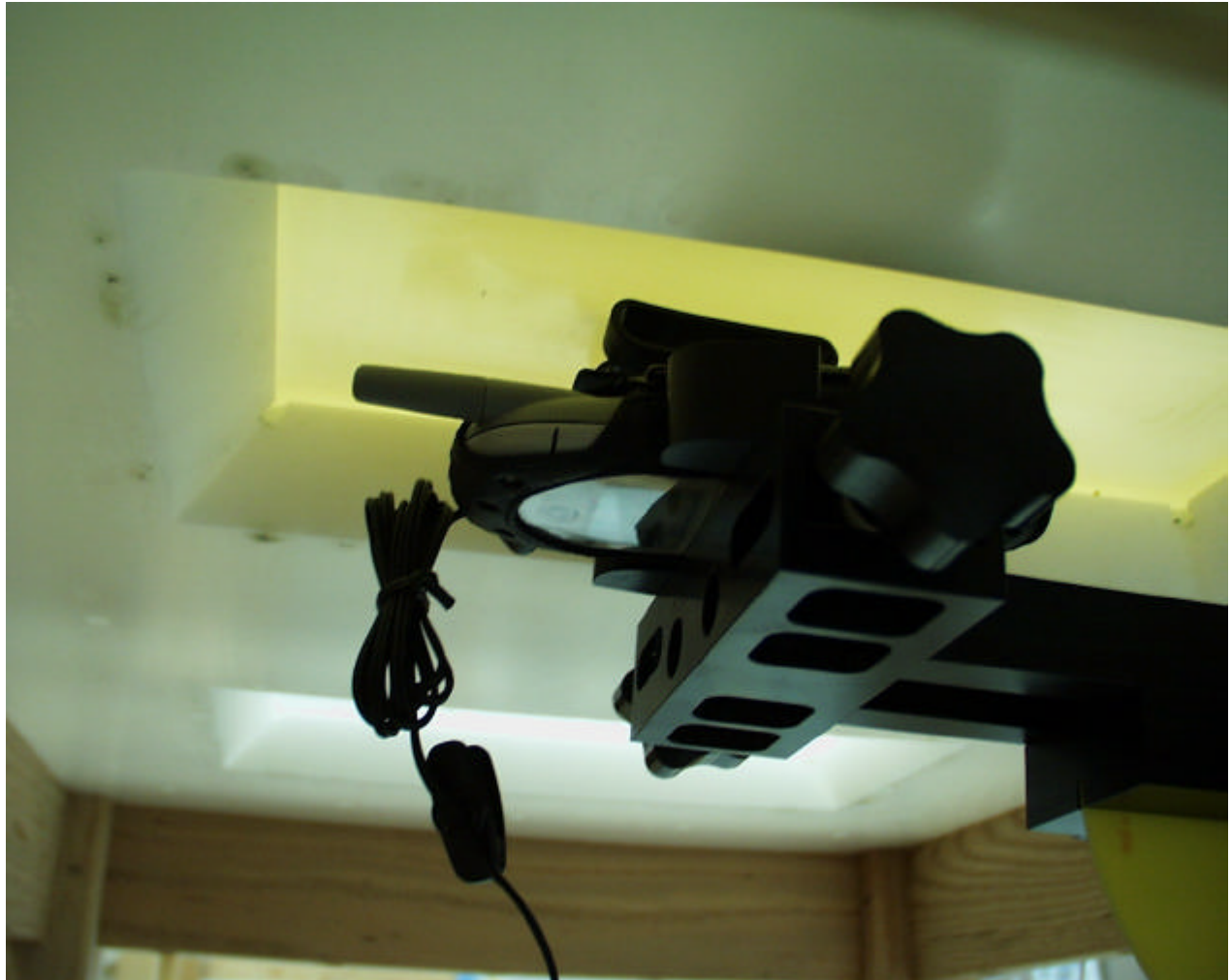
Figure 15. Phone Placed in Body Worn Testing Configuration with Leather Pouch / Belt Clip and Headset Attached
