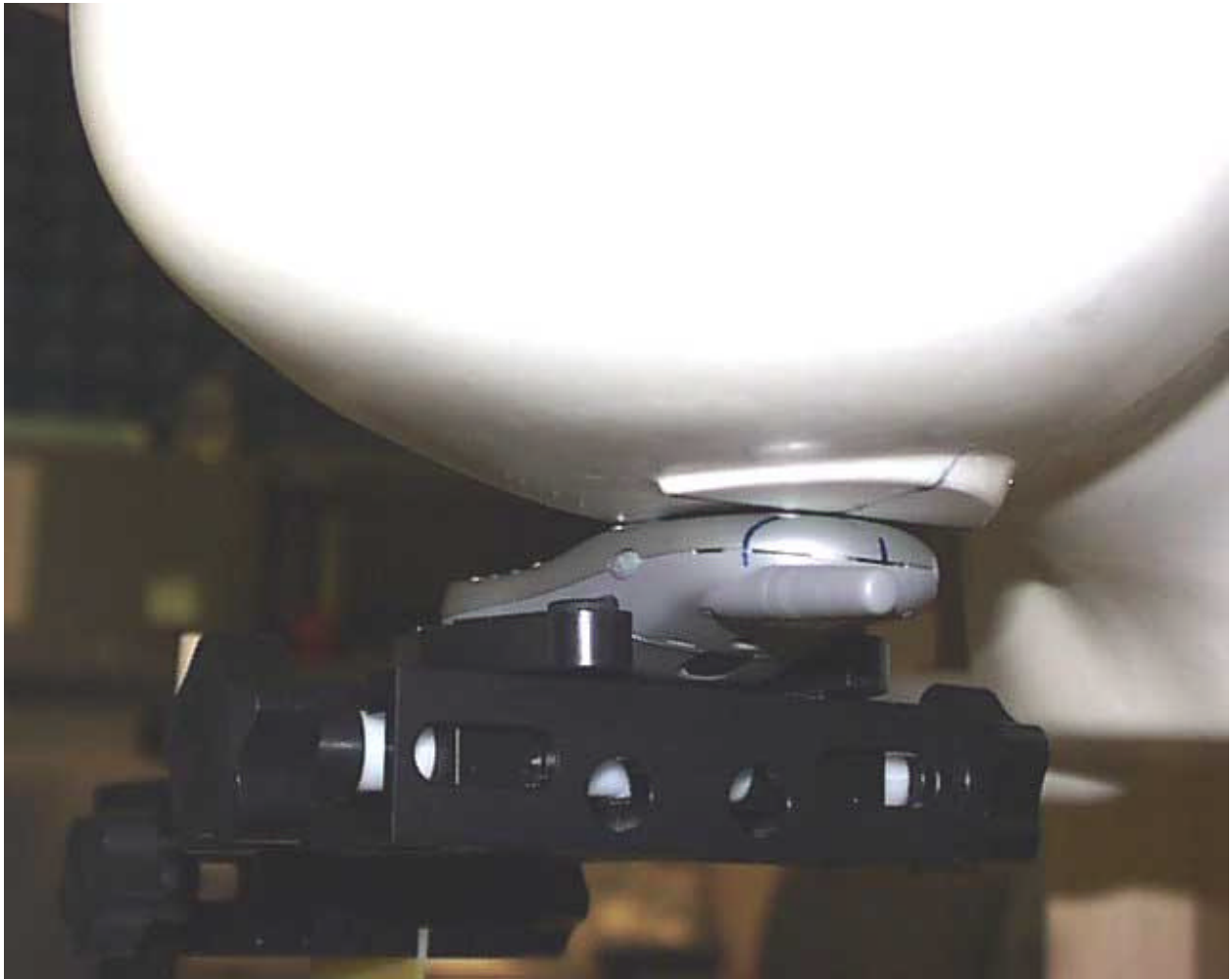
Figure 11. Top of Phone Seen in Cheek Touch Testing Configuration
