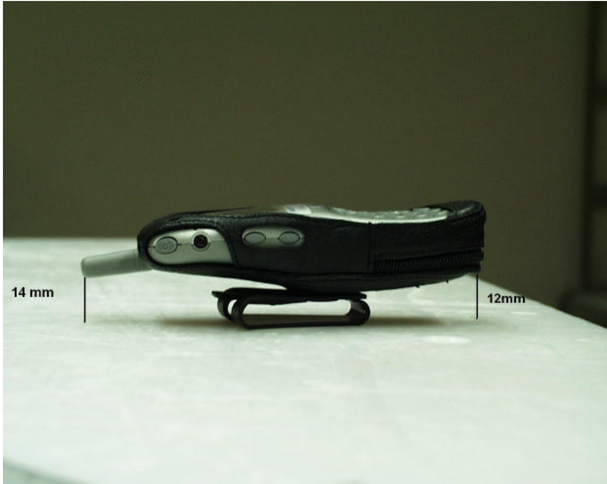
Figure 10. Separation Distance Provided from Leather Pouch
