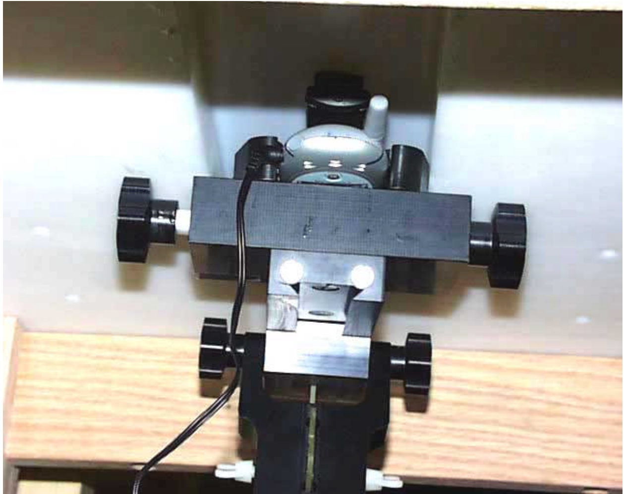
Figure 15. Phone Placed in Body Worn Testing Configuration with Plastic Belt Clip and Headset Attached
