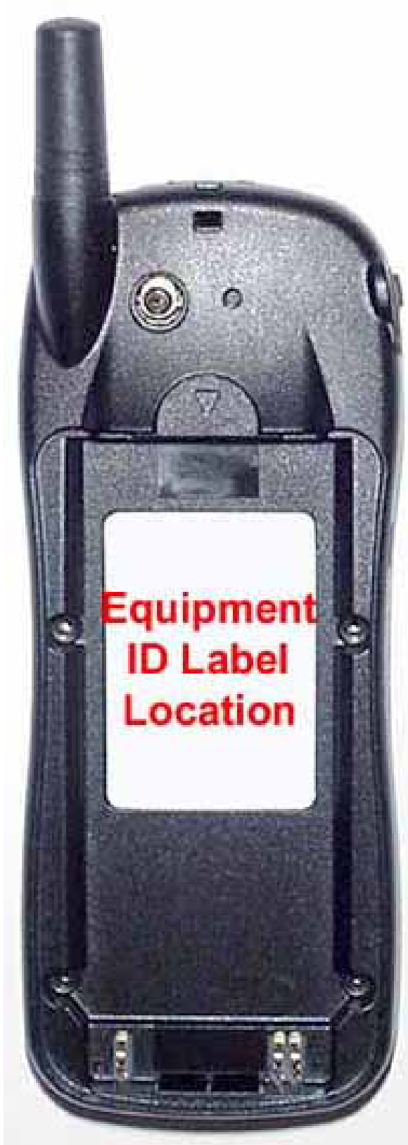
Rear View, with Battery Removed to Show Equipment ID Label
