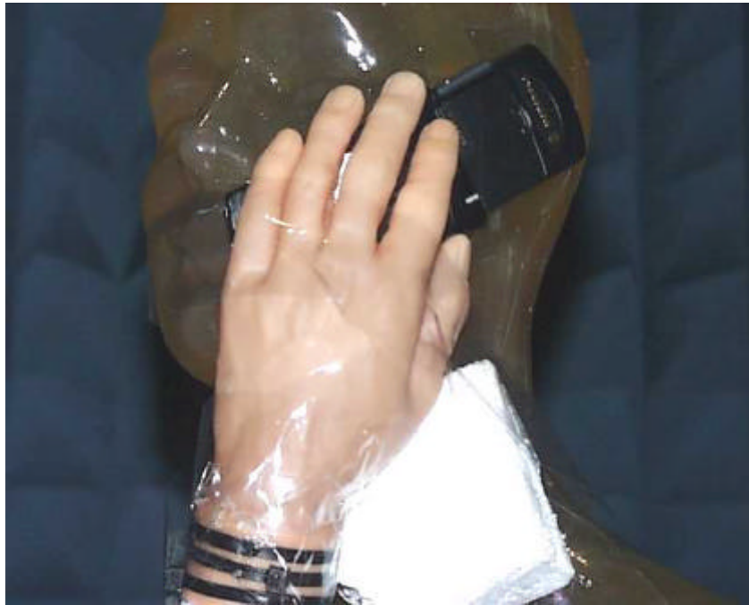
Figure 7. Simulated Hand Against Phantom Head.
