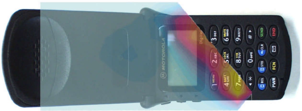
Figure 6. 1900MHz Contour Plot Overlaid on Face of Phone.
