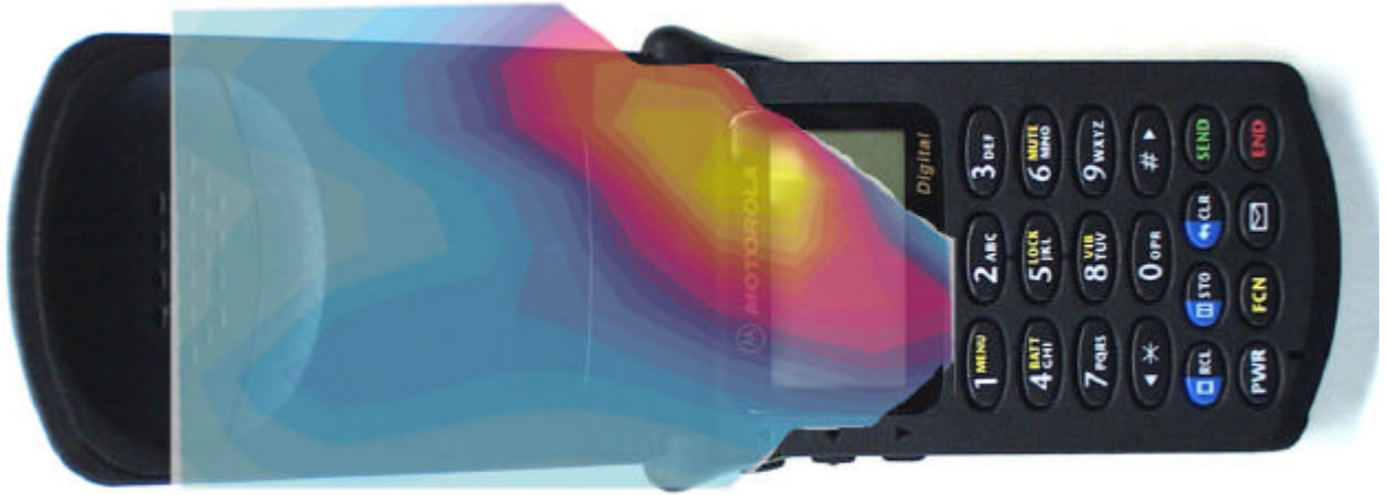
Figure 5. 800MHz Contour Plot Overlaid on Face of Phone.
