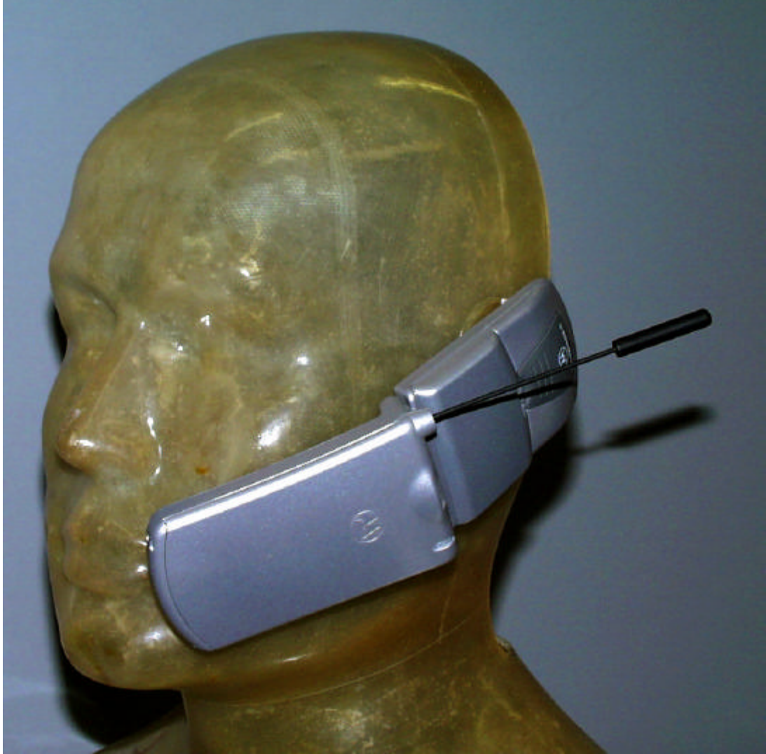
Figure 3. Phone against side of Phantom Head.
