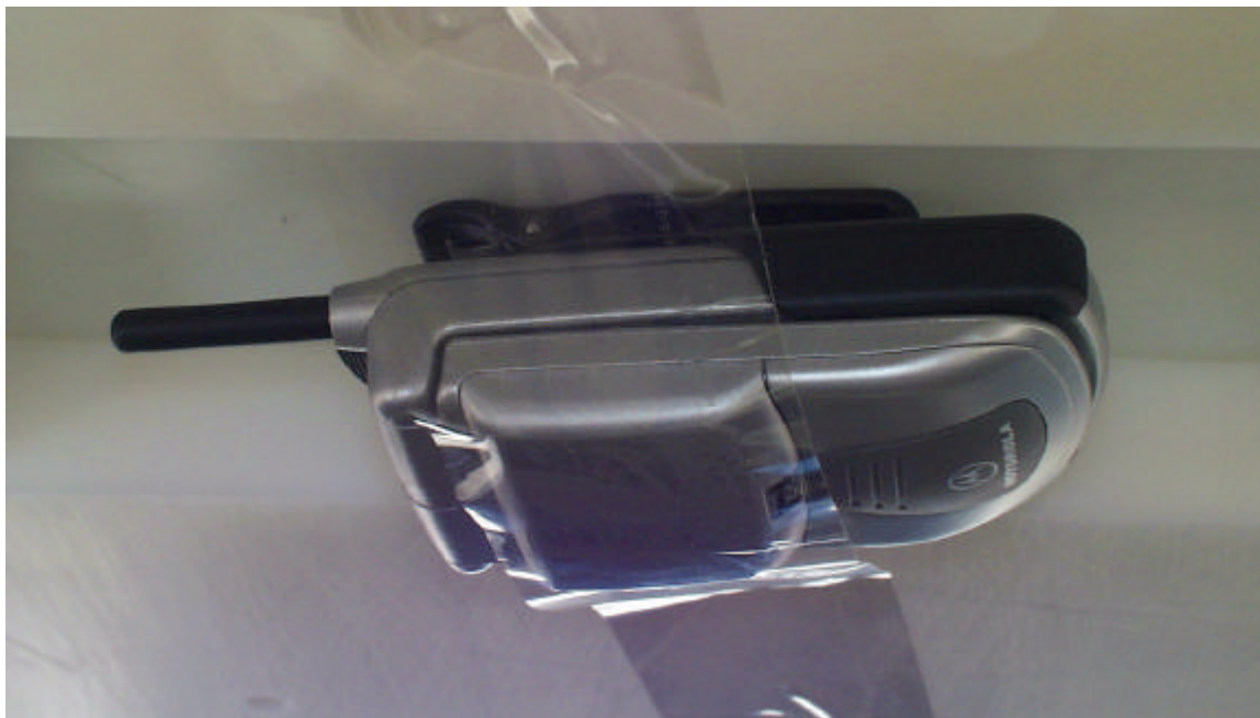
Figure 9. Phone In "Normal" Belt Clip Against Phantom
