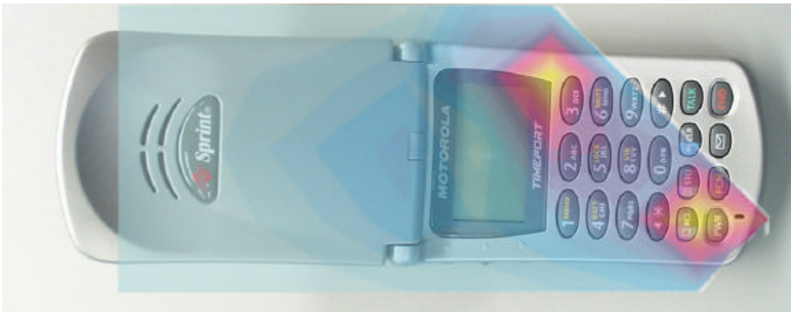
Figure 6. 1900MHz Contour Plot Overlaid on Face of Phone with Antenna Retracted.
