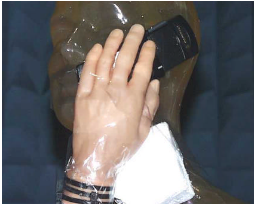
Figure 7. Simulated Hand Against Phantom Head.
