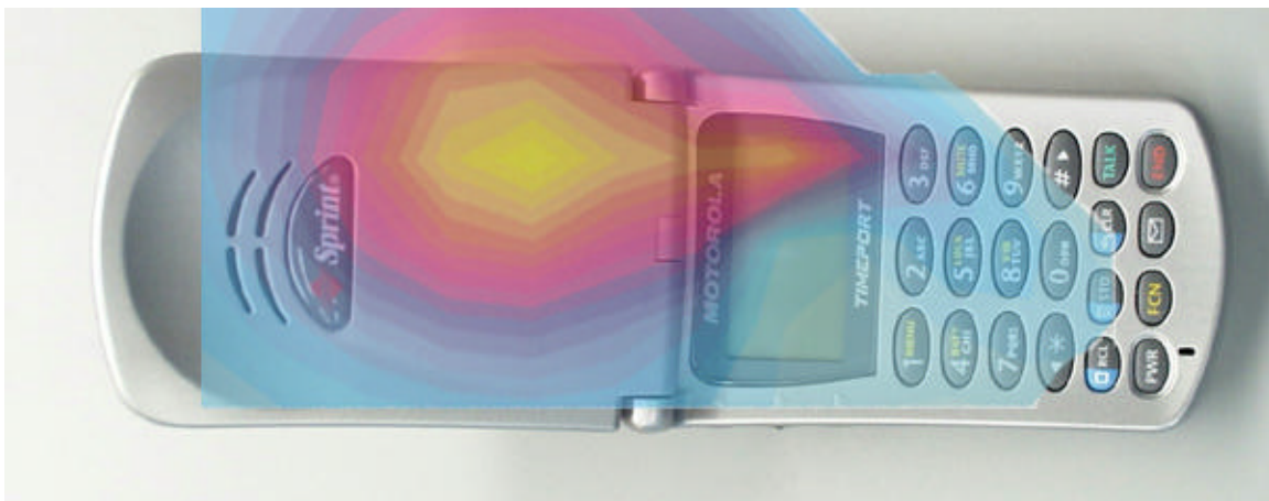
Figure 5. 800MHz Contour Plot Overlaid on Face of Phone with Antenna Extended.
