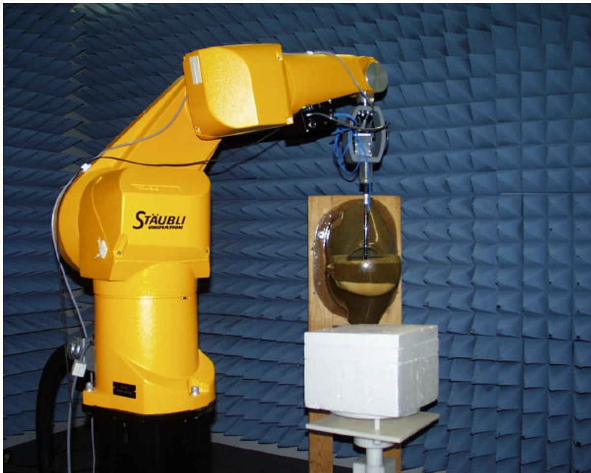
Figure 3. Dasy™ System used for measurements
