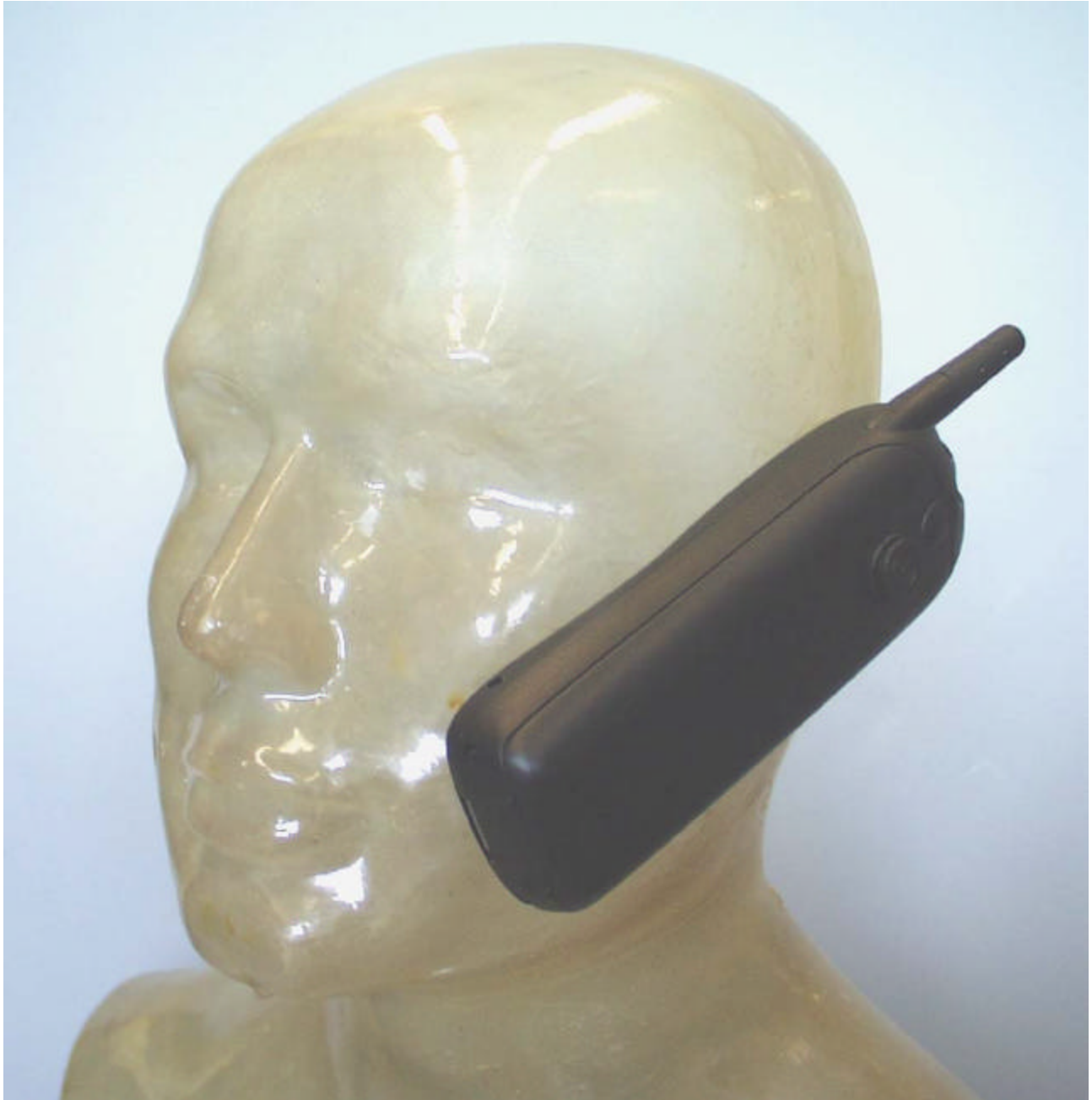
Figure 2. Phone Against Head in Normal Use Position
