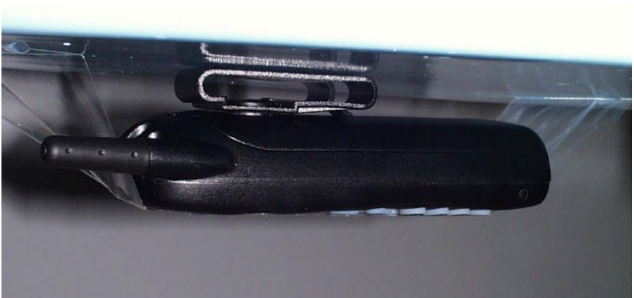
Figure 6. Phone In Supplied Belt Clip Against Phantom
