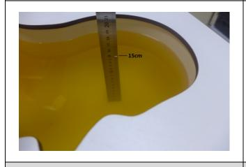
Photo 5: Tissue Simulant Liquid for Head 2600
