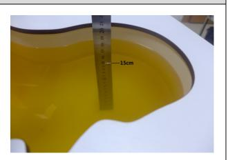
Photo 3: issue Simulant Liquid for Head 1900
