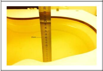
Photo 1: Tissue Simulant Liquid for Head 835
