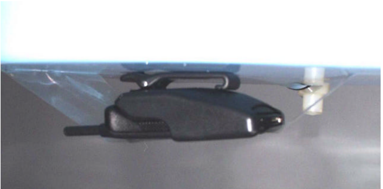
Figure 1. Phone In Supplied Belt Clip Against Phantom
