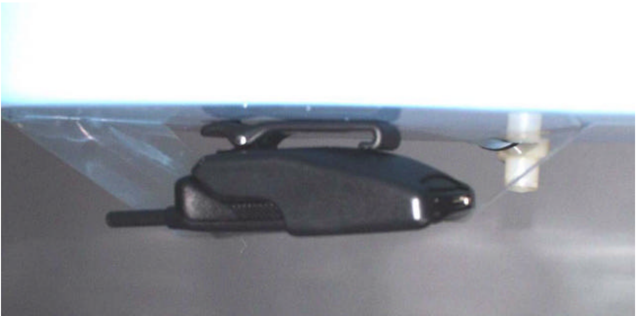
Figure 1. Phone In Supplied Belt Clip Against Phantom
