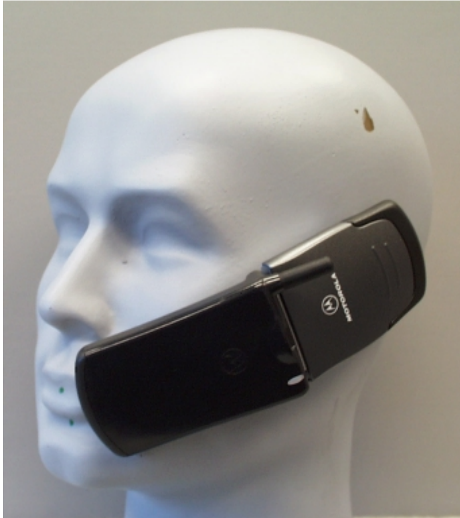
Figure 2. Phone Against Head in Normal Use Position
