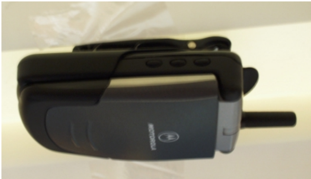
Figure 4. Phone In Supplied Belt Clip Against Phantom
