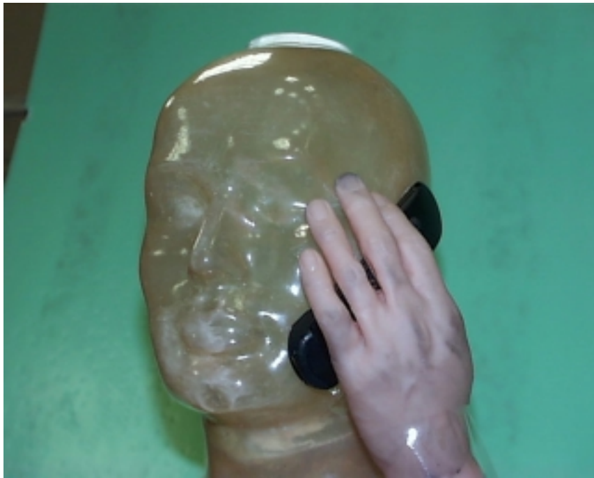
Figure 4. Simulated Hand Against Phantom Head.
