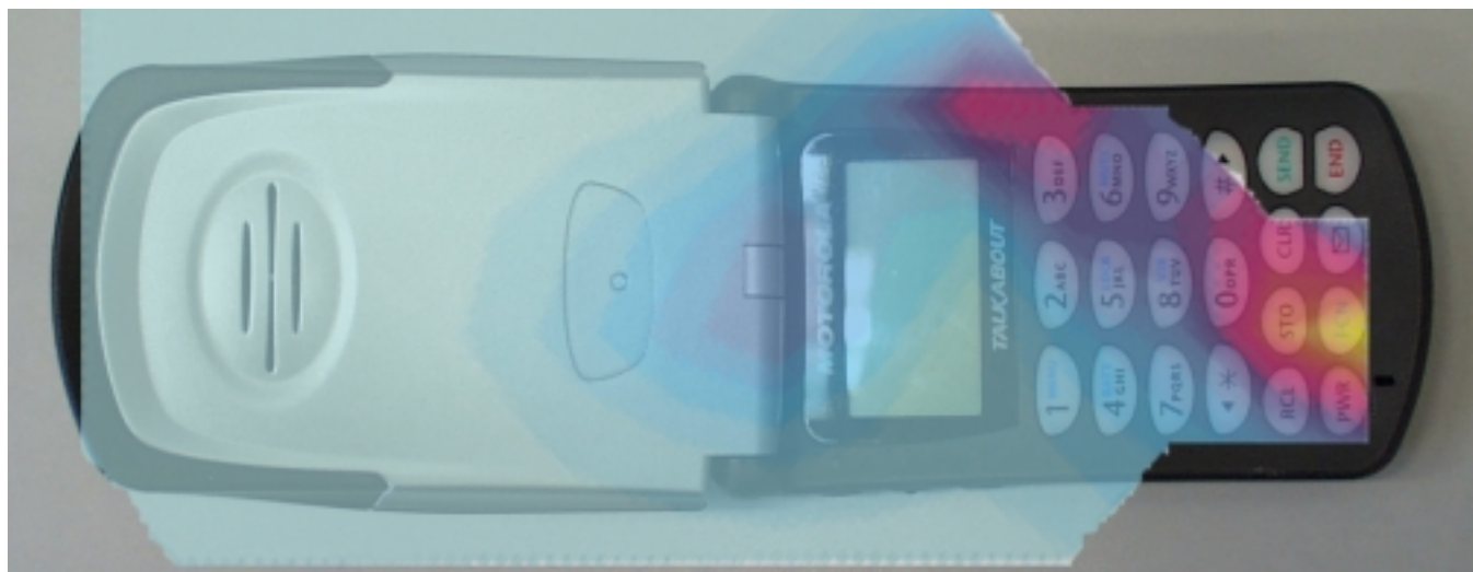
Figure 3. Phone with 1900MHz TDMA Contour Plot Overlay
