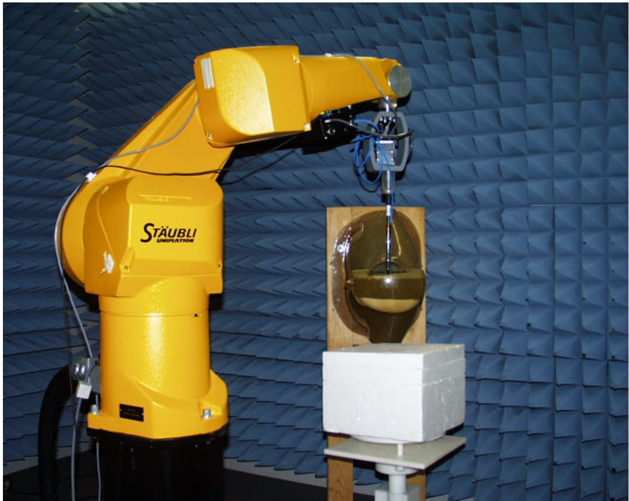
Figure 3. Dasy™ System used for measurements
