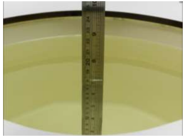
Fig 11.2 Photo of Liquid Height for Body SAR
