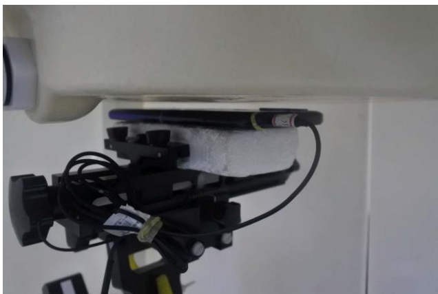
Back with handset 1, Test Separation 5 mm
