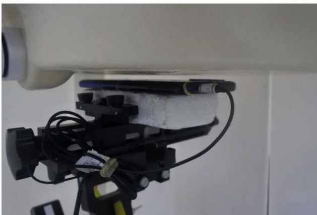
Back with handset 2, Test Separation 5 mm
