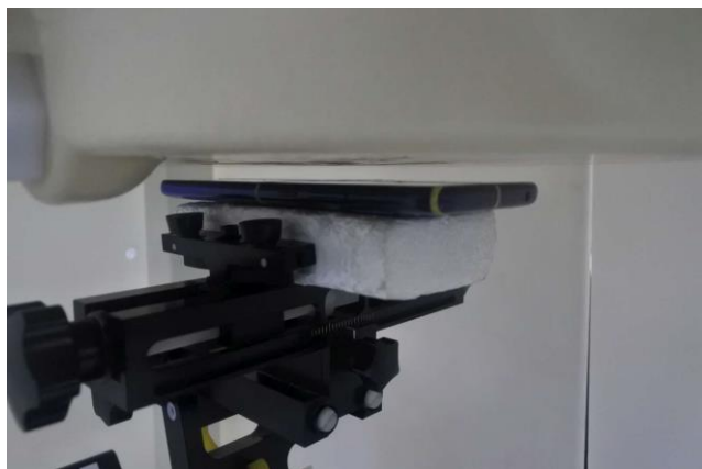
Front, Test Separation 5 mm
