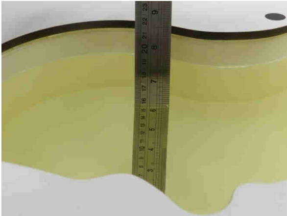
Fig 11.1 Photo of Liquid Height for Head SAR
