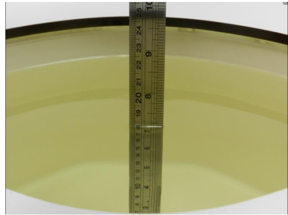
Fig 11.2 Photo of Liquid Height for Body SAR
