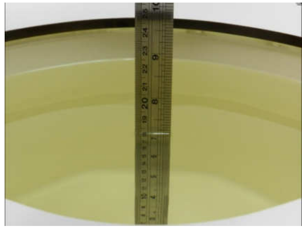
Fig 10.2 Photo of Liquid Height for Body SAR
