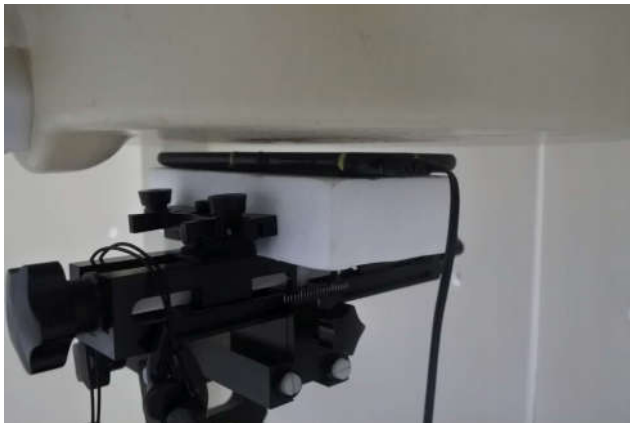
Front with handset, Test Separation 5 mm
