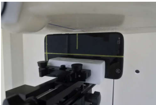
Right Side, Test Separation 5 mm
