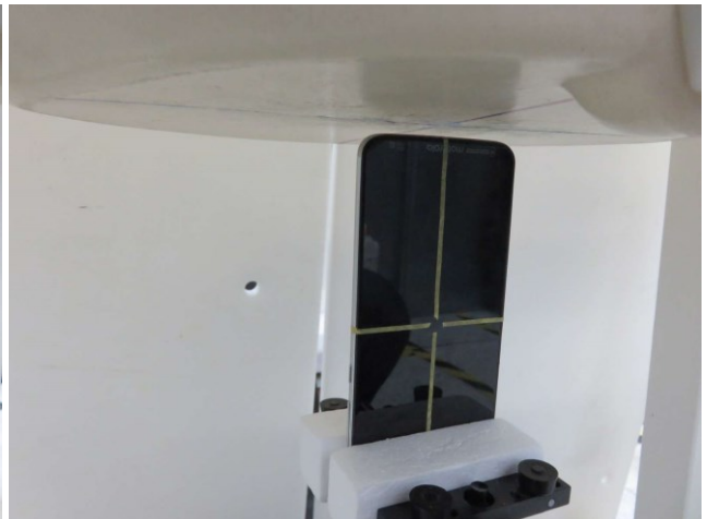
Bottom Side, Test Separation 5 mm
