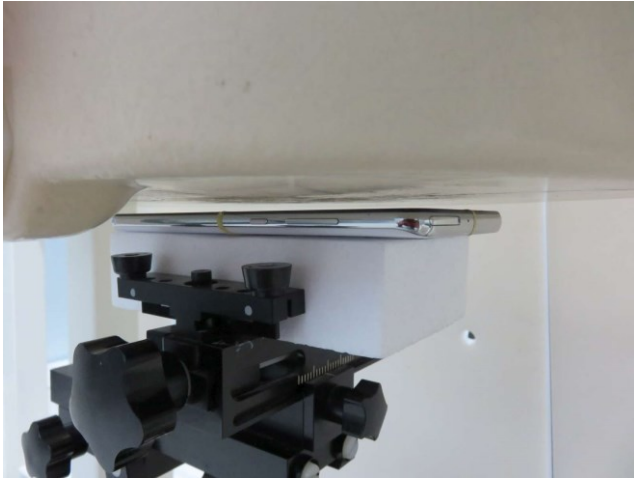
Front, Test Separation 5 mm
