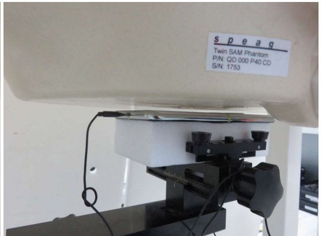
Back with handset, Test Separation 5 mm
