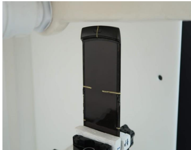
Bottom Side, Test Separation 5 mm
