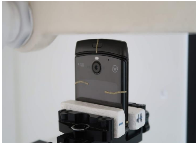
Bottom Side, Test Separation 5 mm
