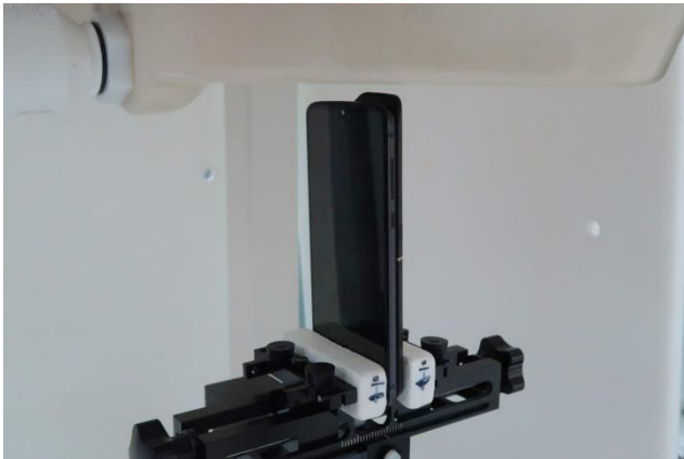
Top Side, Test Separation 5 mm
