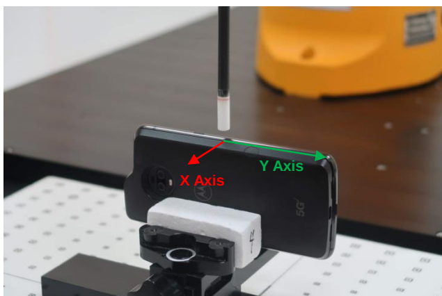
Left Side, Probe sensor to EUT surface distance 5mm
