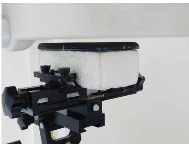
Back, Test Separation 5 mm
