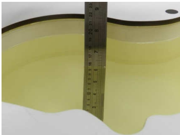
Fig 10.1 Photo of Liquid Height for Head SAR
