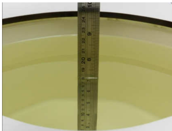
Fig 10.2 Photo of Liquid Height for Body SAR
